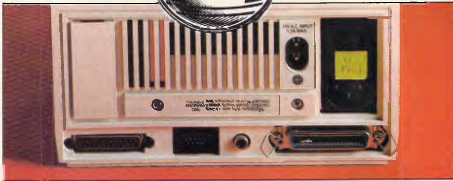
The back features a two-pin monochrome monitor socket
